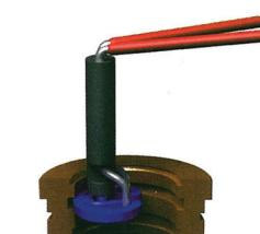
4. Put the seal in the groove
