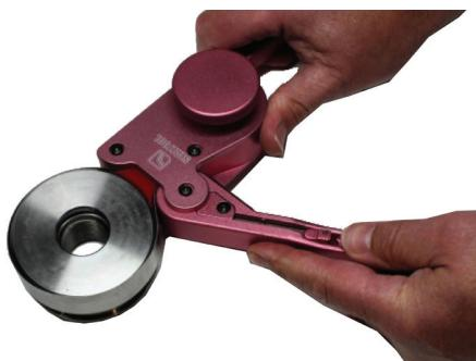
5. Calibrate the seal using the tool **19SEAL CLASPER**.
